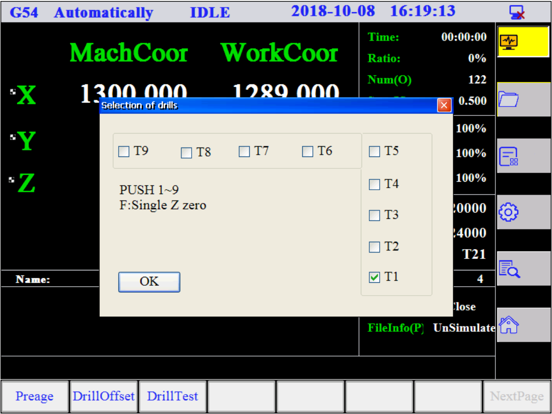
Figure 13-18 Cylinder Tool Changing XY Offset Setting
